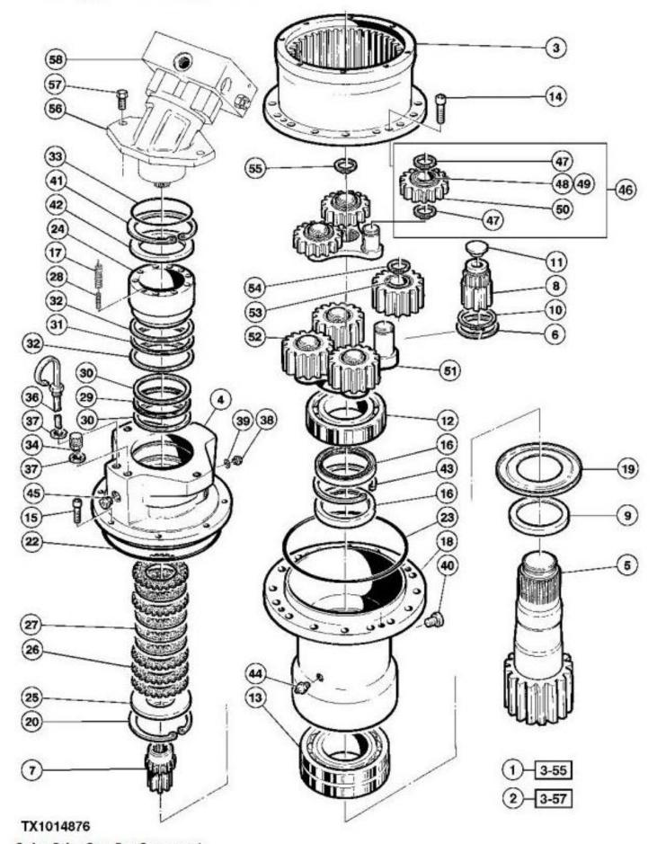
Swing Drive Gear Box Components
