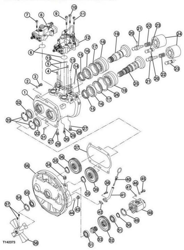
Hydraulic Pump and Pump Drive Gear Case (1 of 2)
