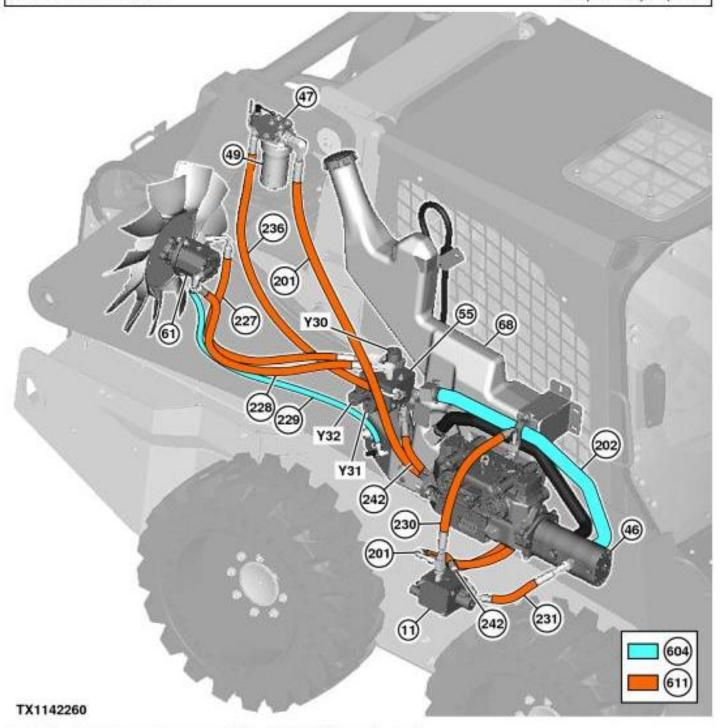
Hydraulic Fan Component Location (S.N. -269401) (reversing fan)
