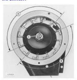
Pickup Finger Contact Points and Shaft
