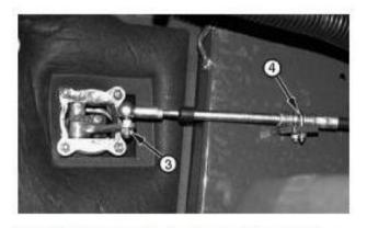
Throttle Cable-To-Accelerator Pedal Connection
