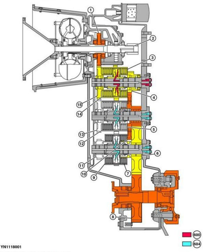
Transmission Operation 1 Gear Forward
