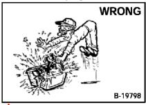
Lead-acid batteries produce flammable and explosive gases.
