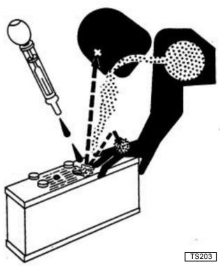
Sulfuric acid in battery electrolyte is poisonous. It is strong enough to burn skin, eat holes in clothing, and cause blindness if splashed into eyes.
