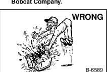
Lead-acid batteries produce flammable and explosive gases. Keep arcs, sparks, flames and liahted tobacco away from batteries.
