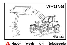
handler with boom up unless boom is held by an approved boom stop. Replace if damaged.
