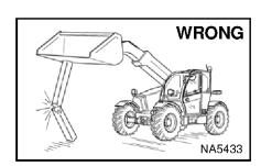
Never work on telescopic handler with boom up unless boom is held by an approved boom stop. Replace if damaged.
