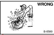
Lead-acid batteries produce flammable and explosive gases.
